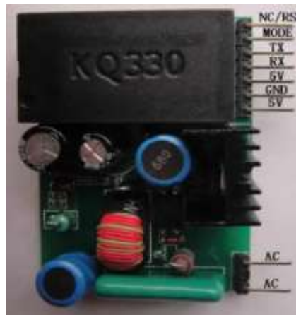
Fig.2. power line carrier KQ330 module
